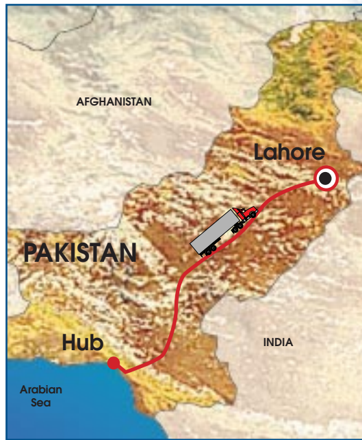
Along with other plant components, BOC Pakistan’s air treatment module (ATM) was transported from Hub to Lahore, Pakistan via truck. The ATM contains the equipment for chilling, dehumidifying, and purifying the process air before it enters the cold box.
