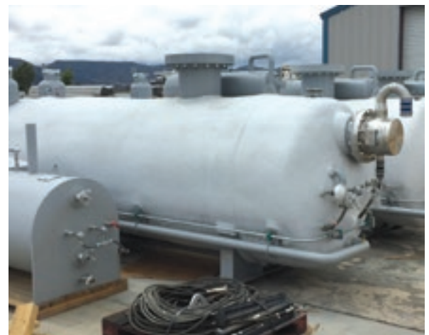
Smaller version of the waterbath vaporizer
