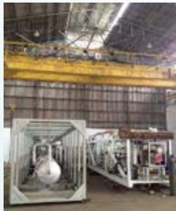
COLD BOX AND WARM END SHIP INSIDE 45 FOOT ISO CONTAINERS, COMPLETE WITH ALL PIPING, INSTRUMENTS, ELECTRICAL AND INSTRUMENTATION
