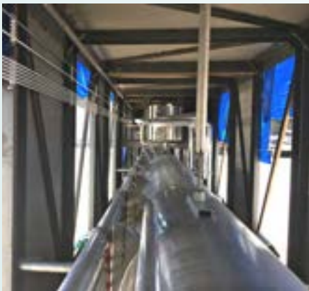
COLD BOX SHIPPED PRE- FABRICATED AND INSULATED WITH PERLITE, NO FIELD ACCESS
