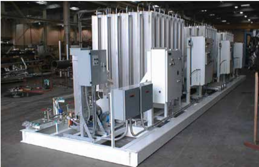
Skidded high pressure ambient vaporizer system
