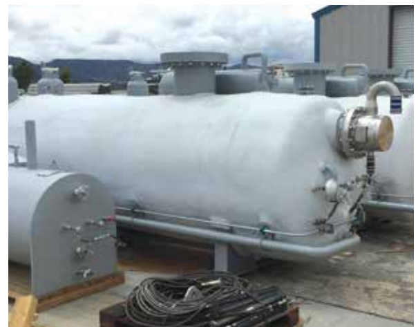
Smaller version of the waterbath vaporizer
