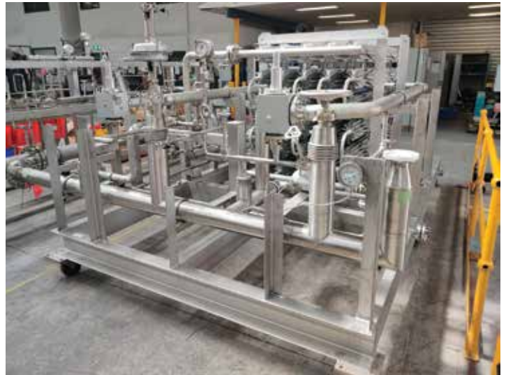
LH 2 Pressure Decant Skid
